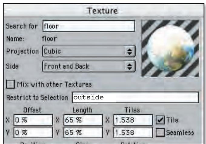
Figure 14: Type the word 'outside' into the Restrict to Selection text box
